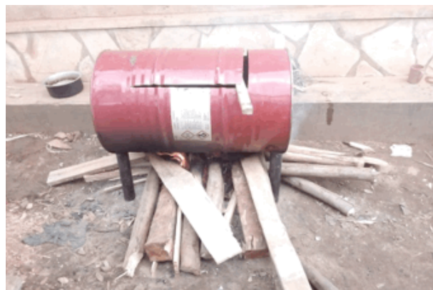
Figure 36: Steam sterilization of rooting media by use of a metallic drum
